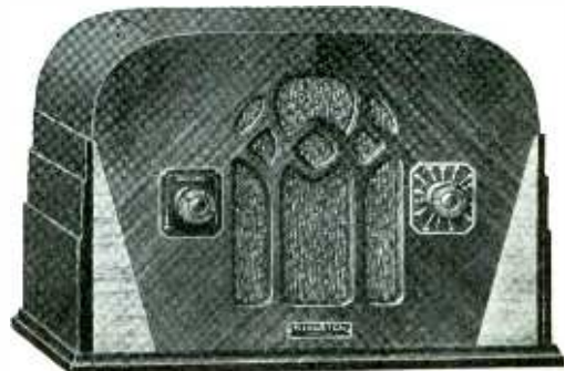
● Model 600A — A six-tube superheterodyne which gives nine-tube performance, by the use of "dual purpose" tubes. High frequency amplifier stage. Six tuned circuits. Specially designed 6½" dynamic speaker. Switch and tone control combined. Tuning range covers standard American band and certain police and amateur stations, 170 to 555 meters. Price $39.95
